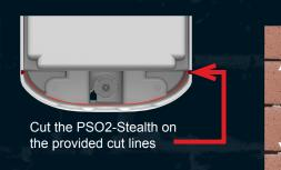
Once optional cut-section is removed, PSO1-Stealth / PSO2-Stealth fits between two bricks making installation simple and easy.
