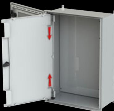
1) To remove or place the inner door in an Allbrox® simply pull the two hinge pins as indicated towards each other.
